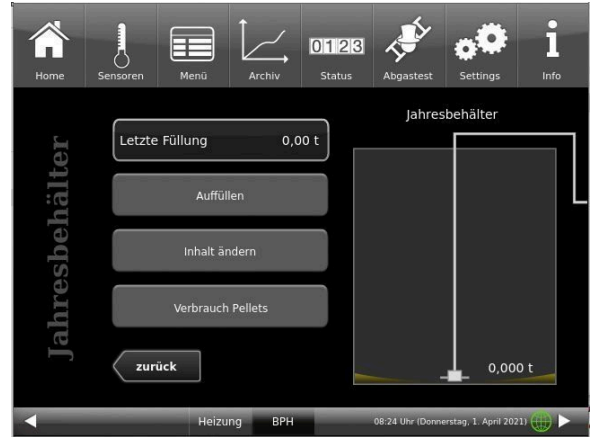
Illustration 9: Display with pellet mole system installed (example with empty annual hopper)
